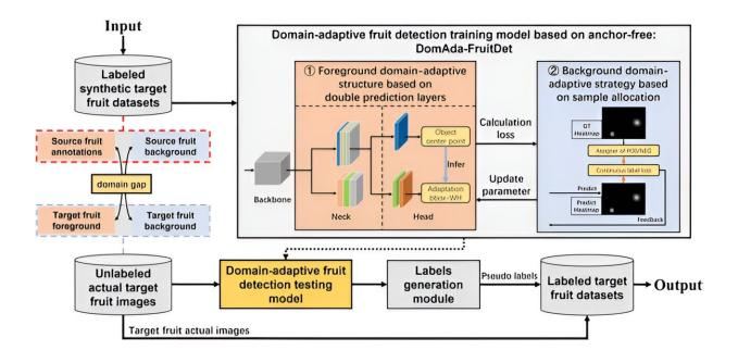
Flowchart for using DomAda-FruitDet to improve the accuracy of the EasyDAM method, with the labeled target domain synthetic fruit dataset as input and the obtained labeled target domain actual fruit dataset as output. Credit: *Plant Phenomics* (2023). DOI: 10.34133/plantphenomics.0135
