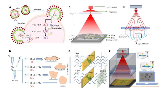
Principle and structure of the online location detection system for virus infection in cells based on lensless diffraction. (A) Change mechanism of cells after virus stress. (B) Schematic diagram of diffraction principles. (C) Principle of the diffraction fingerprint formed by the optical path in the diffraction process. (D) Schematic diagram of cell morphological changes at different times after virus stress. (E) Effect of different morphologies on the light path. (F) Schematic
