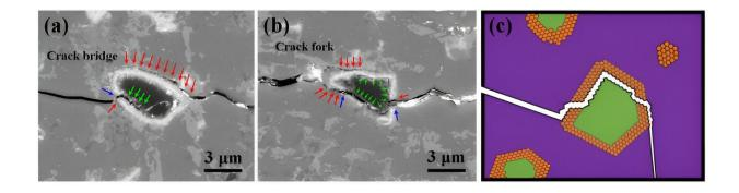
(a, b) BSE images of polished surface with cracks of Al<sub>2</sub>O<sub>3</sub>-B<sub>4</sub>C@TiB<sub>2</sub> composite ceramics. (c) Schematic diagram for crack propagation. Credit: Journal of Advanced Ceramics, Tsinghua University Press
