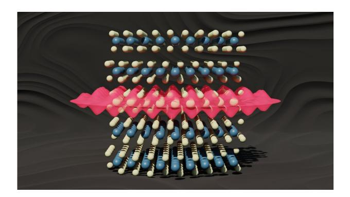
Atoms of a tantalum disulfide (TaS2) crystal with a 2D endotaxial layer in the center. The pink cloud represents the charge density wave, a clumped pattern of electrons, surrounding the 2D layer. Credit: Hovden Laboratory
