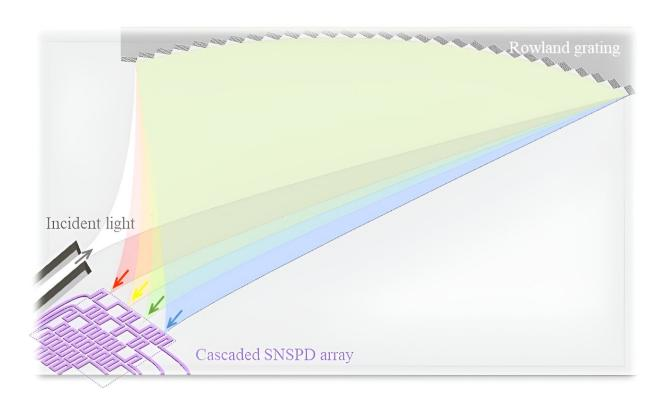
Photon-counting reconstructive spectrometer. Credit: Advanced Devices & Instrumentation (2023). DOI: 10.34133/adi.0021
