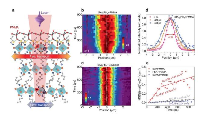
Exciton transport in exfoliated (BA)<sub>2</sub>PbI<sub>4</sub> RPP flakes encapsulated by coverslip and PMMA. Credit: *Nature Communications* (2024). DOI: 10.1038/s41467-024-45740-y
