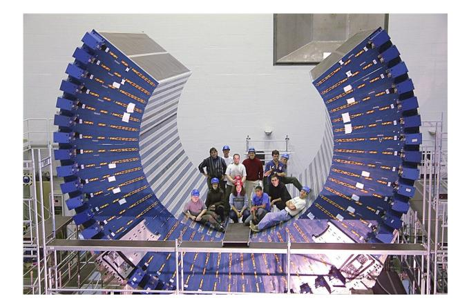
The tile calorimeter under construction, an iron detector at the center of ATLAS weighing nearly 4,000 metric tons, which serves as a useful volume for neutrino
