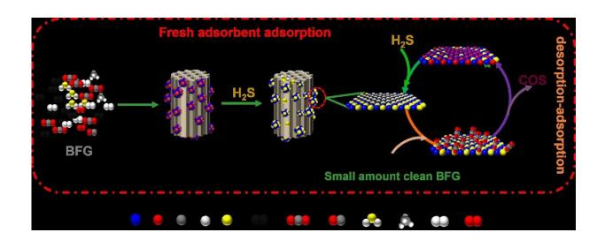
$H_2S$  removal and regeneration mechanism of  $NH_3$ –CuO/13X-3 adsorbent. Credit: Erping Cao, et al.
