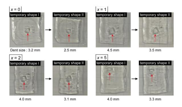
Photographs of the hydrogels with temporary shapes I and II. Credit: *Advanced Materials Technologies* (2024). DOI: 10.1002/admt.202301598
