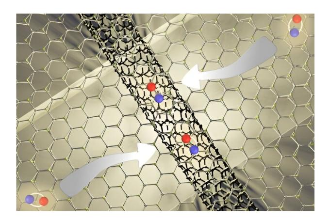
An atomically thin flake of tungsten diselenide acts as a reservoir for excitons, which are made up of electrons (red) and holes (blue). These excitons quickly pass into a narrow carbon nanotube suspended over a trench. Credit: RIKEN Nanoscale Quantum Photonics Laboratory
