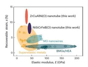
"Our research introduces a nano-oxide engineering approach for low-dimensional metallic glasses. The morphology of nano-oxides within metallic-glass nanotubes and nanosheets can be manipulated by adjusting the oxide concentration, ranging from isolated dispersions to a connected network," said Professor Yang. Credit: City University of Hong Kong
