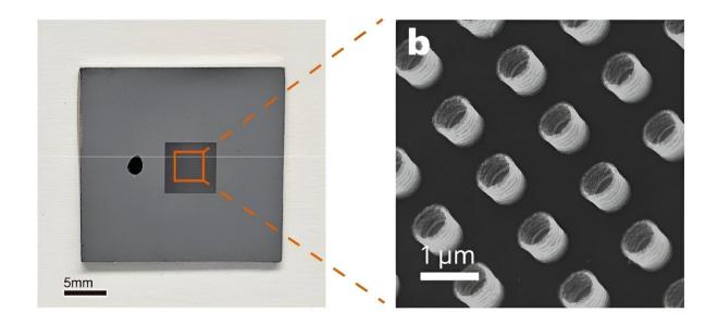
(Left) Photo of metallic-glass nanotubes fabricated on silicon and (right) a scanning electron microscopy image of the metallic-glass nanotubes. Credit: Professor Yang Yong's research group / City University of Hong Kong
