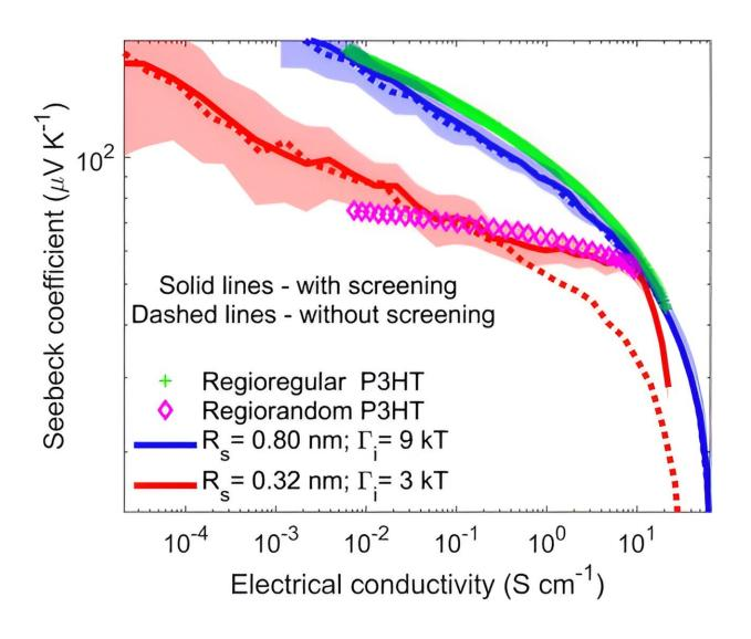
Seebeck coefficient against electric conductivity measurements of RR and RRa-P3HT doped with iodine and measured while dedoping. We took Rd= 0.21 nm
