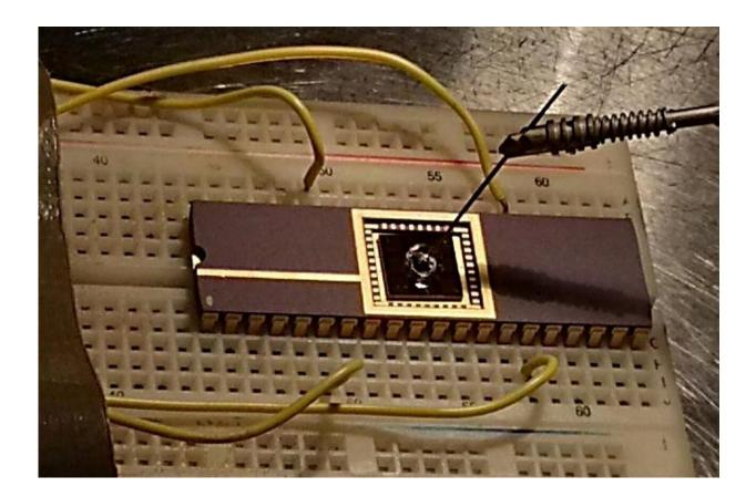
Experimental setup of the device detecting lead ions in a drop of water. Credit: Bandaru Lab/UC San Diego
