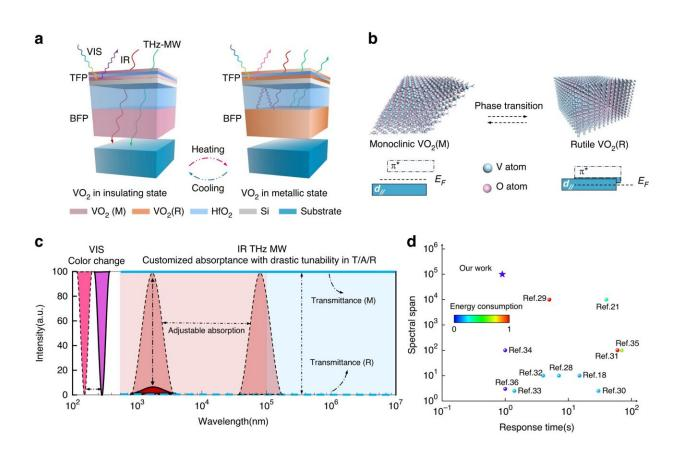
Schematic of proposed system with its operating principle. Credit: *Light: Science* & *Applications* (2024). DOI: 10.1038/s41377-024-01400-w
