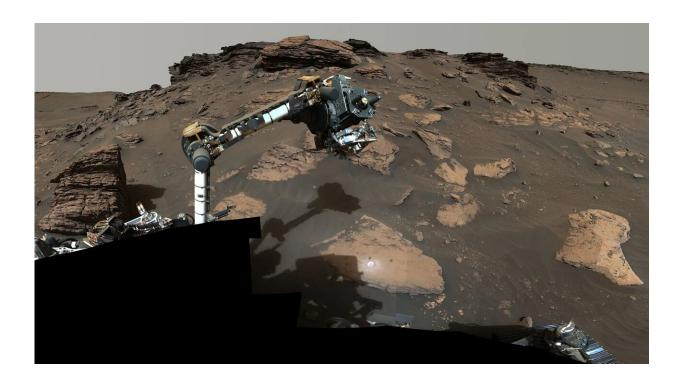
NASA's Perseverance puts its robotic arm to work around a rocky outcrop called "Skinner Ridge" in a set of images captured in June and July 2022 by the rover's Mastcam-Z camera system. SHERLOC is mounted on the end of the arm. NASA/JPL-Caltech/ASU/MSSS
