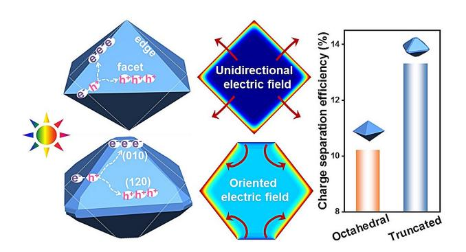
Tailoring morphology symmetry of  $BiVO_4$  photocatalyst from octahedral to truncated octahedral crystals leads to the quite different separation of photogenerated charges and a significantly improved charge separation efficiency. The built-in electric field for driving photogenerated charge separation is considered to be modulated by tuning the morphology symmetry. Credit: Science China Press
