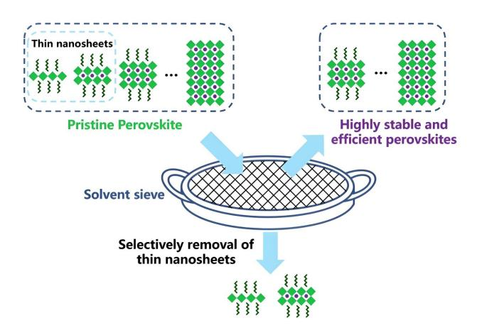
The solvent sieve method for high-performance PeLEDs. Credit: NIMTE
