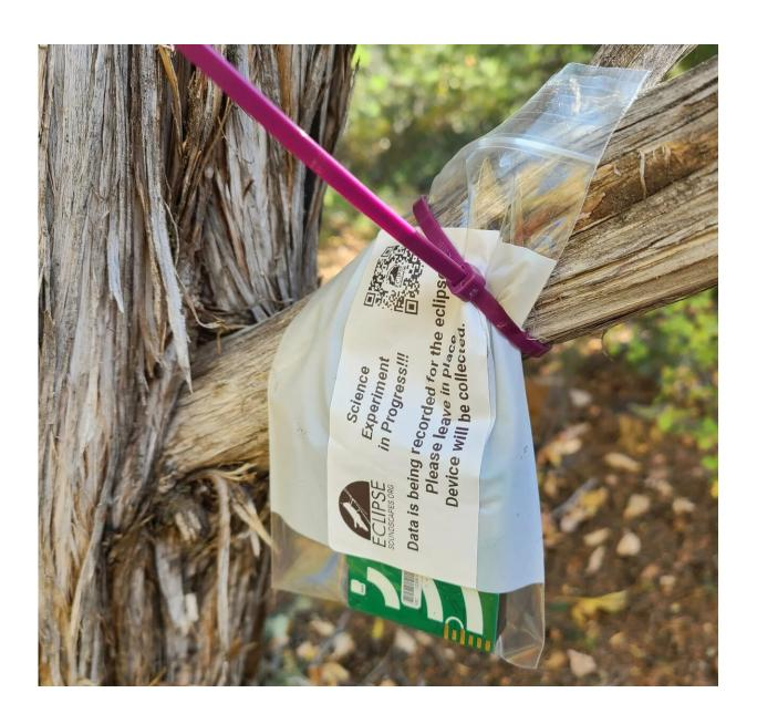
An AudioMoth device hangs from a tree branch, ready to capture the sounds of
