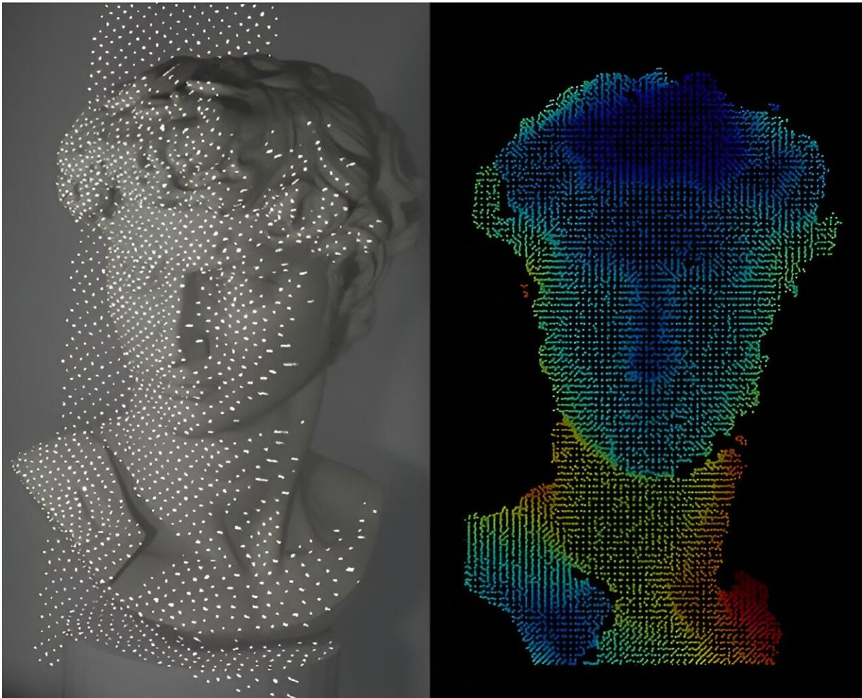
A new lens-free and compact system for facial recognition scans a bust of Michelangelo's David and reconstructs the image using less power than existing 3D surface imaging systems. Credit: *Nano Letters* (2024). DOI: [10.1021/acs.nanolett.3c05002](https://doi.org/10.1021/acs.nanolett.3c05002)
