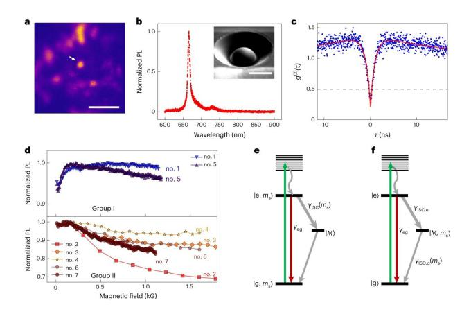
Optical properties of GaN defects. **a**, PL image of an isolated defect (no. 2), indicated by an arrow, and its surroundings. Scale bar, 2  $\mu$ m. **b**, Optical spectrum of defect no. 2. The inset shows a scanning electron microscope image of a solid immersion lens carved around the defect. Scale bar, 4  $\mu$ m. **c**, Second-order photon autocorrelation  $g^{(2)}(\tau)$  of defect no. 2, where  $\tau$  is the delay. The zero-delay autocorrelation  $g^{(2)}(0) = 0.3$
