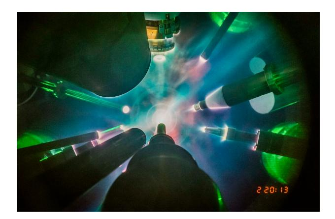
A a view from inside the OMEGA target chamber during a direct-drive inertial fusion experiment at the University of Rochester's Laboratory for Laser Energetics. Scientists fired 28 kilojoules of laser energy at small capsules filled with deuterium and tritium fuel, causing the capsules to implode and produce a plasma hot enough to initiate fusion reactions between the fuel nuclei. The temperatures achieved at the heart of these implosions are as high as 100 million
