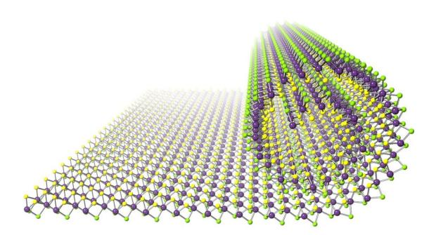
By replacing the atoms on one side of the nanosheet with a different element, the team have realized a nanosheet that can spontaneously roll into a scroll when detached from its substrate. Credit: Tokyo Metropolitan University
