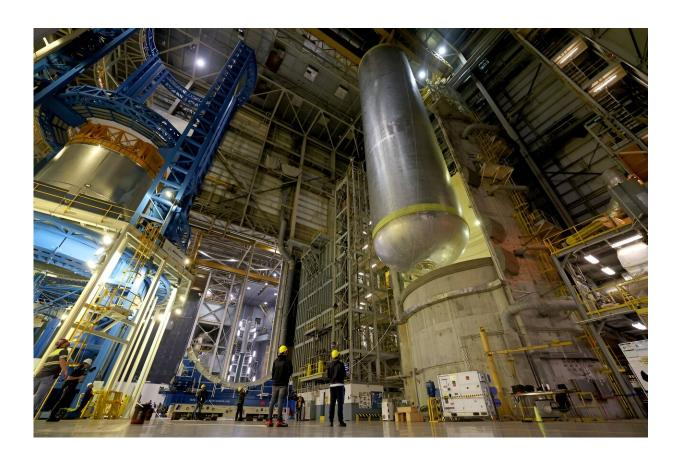
All the major structures that will form the core stage for NASA's SLS (Space Launch System) rocket for the agency's Artemis III mission are structurally complete. Technicians finished welding the 51-foot liquid oxygen tank structure, left, inside the Vertical Assembly Building at NASA's Michoud Assembly Facility in New Orleans Jan. 8. The liquid hydrogen tank, right, completed internal cleaning Nov. 14. Credit: NASA/Michael DeMocker
