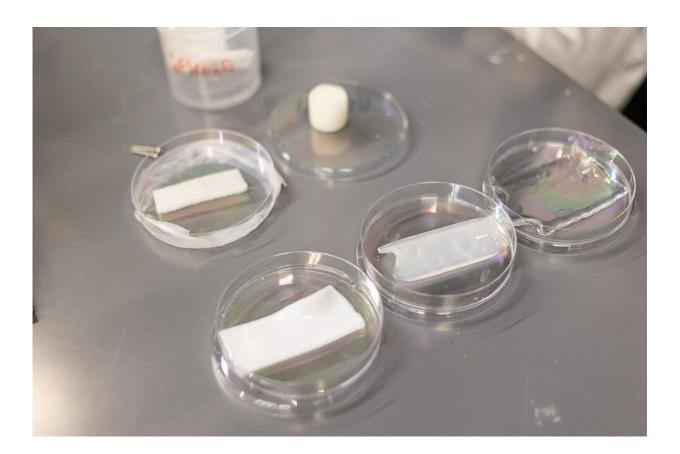
Thermo-responsive polymer composites are shown in Dr. Shuang (Cynthia) Cui's lab. The polymer can make air conditioning more energy efficient by separating the dehumidification and heat removal processes and improving the most energy-consuming steps. Credit: University of Texas at Dallas
