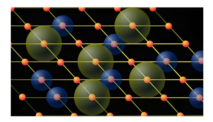
Illustration of a quantum simulator with atoms trapped into a square lattice with lasers. The small spheres at the corners are atoms in their lowest energy state. The ones inside a blue sphere are exited (higher in energy) by the first laser, the ones inside yellow spheres are excited by the second laser (even more higher in energy). Credit: TU Delft
