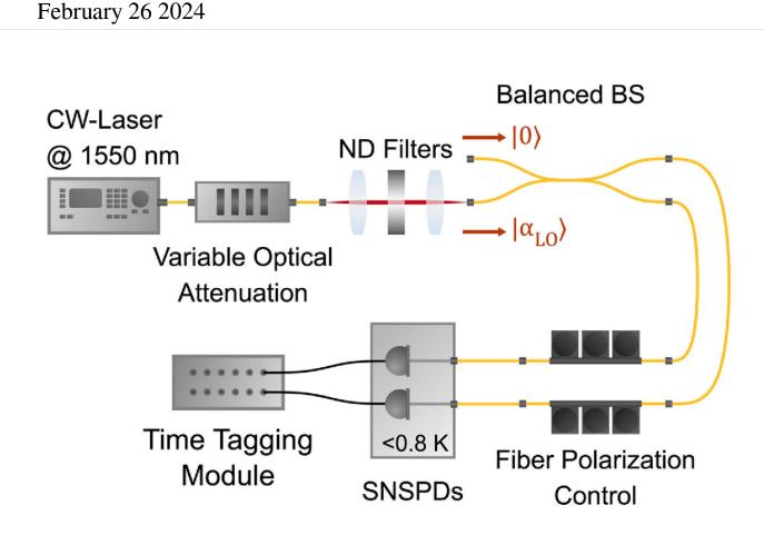
Setup used to investigate the linearity of two SNSPDs in terms of the local oscillator photon flux. The field of the vacuum state is interfered with a continuous-wave (CW) local oscillator on a balanced fiber beam splitter. Credit: *Optica Quantum* (2023). DOI: 10.1364/OPTICAQ.502201
