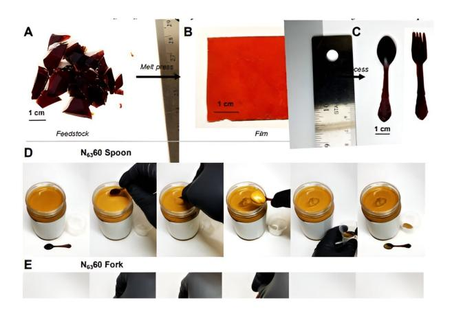
Applications from a single feedstock. A, Batch of as-cast, dried  $N_{63}$ . B, Freestanding film of  $N_{63}$ . C,  $N_{63}60$  spoon and fork. D, Demonstration of  $N_{63}60$ as a rigid spoon to scoop peanut butter. E, Demonstration of  $N_{63}60$  as a rigid fork to pick up a piece of cheese. F, Demonstration of  $N_{63}110$  as a pressuresensitive adhesive. G, Demonstration of  $N_{63}60$  immediately failing as an adhesive. Credit: *Science* (2024). DOI: 10.1126/science.adi5009
