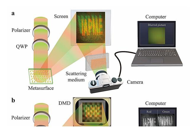
a. Schematic diagram of the commercial camera imaging of the superimposed dual-color images reconstructed by the metasurface in the presence of a scattering medium. b. Schematic diagram of the DIP-SPD single-pixel imaging of the superimposed dual-color images reconstructed by the metasurface in the presence of a scattering medium. QWP: quarter-wave plate; DMD: digital micromirror device. Credit: *Light: Science & Applications* (2023). DOI:
