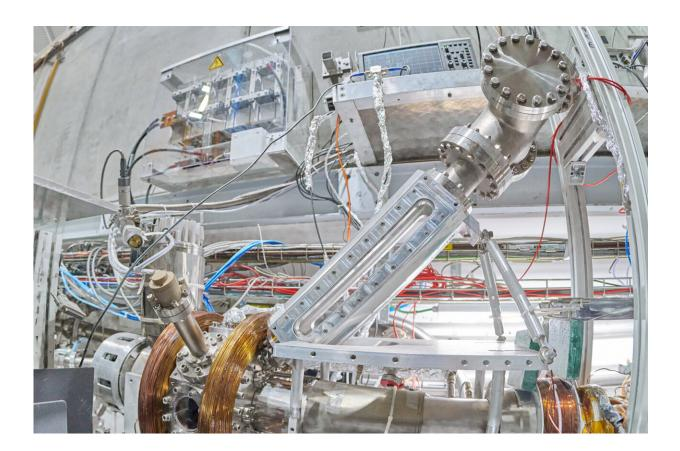
The set-up used by the AEgIS team to laser-cool positronium. Credit: CERN
