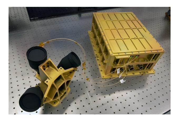
Navigation Doppler Lidar is a guidance system that uses laser pulses to precisely measure velocity and distance. NASA will demonstrate NDL's capabilities in the lunar environment during the IM-1 mission. Credit: NASA/David C. Bowman
