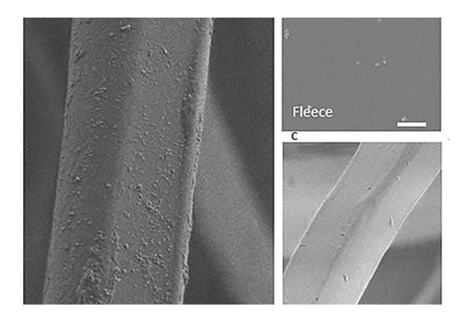
The nanoparticles on the surface of the fleece fiber are visible under a scanning electron microscope (a). The particles detach during washing (b), so that after four washes there are hardly any left. Credit: Empa
