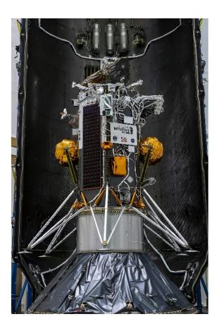
This handout picture from NASA shows the Nova-C lunar lander encapsulated within the fairing of a SpaceX Falcon 9 rocket in preparation for launch.
