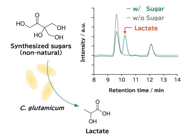
Fig. 2. Lactate fermentation using chemically synthesized sugars as the substrate Credit: ChemBioChem 2024, 25, e202300760. Copyright Wiley-VCH GmbH
