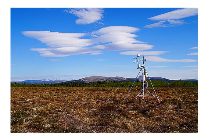
A view of an eddy covariance tower, capable of measuring the release of greenhouse gases, located in Alaska. Credit: Sigrid Dengel
