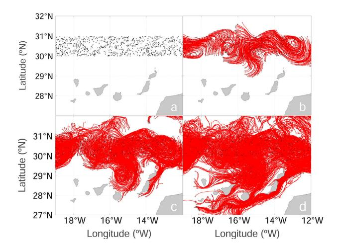
Simulation of trajectories of microplastic particles released into the North Atlantic Ocean after 0 days (a), 12 days (b), 38 days (c) and 76 days (d). Credit: Credit: *Frontiers in Marine Science* (2024). DOI: 10.3389/fmars.2024.1314754
