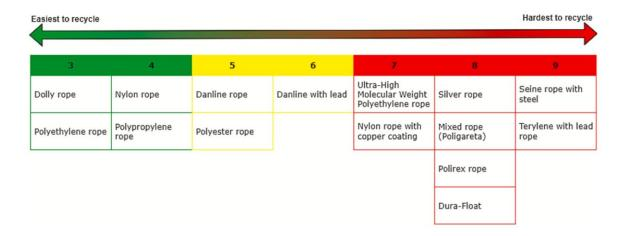
Most of the ropes sold to fishermen in Norway are almost impossible to recycle in a profitable way. New research from NTNU shows that only a third of them are suited for recycling. Credit: NTNU
