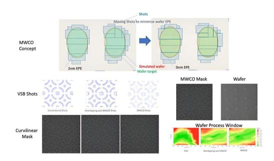
Concept of mask/wafer co-optimization by moving the shot with mask and wafer double simulation to minimize wafer error. VSB shot configurations and its corresponding pattens on mask. MWCO mask and its wafer print. Wafer Process Windows shows MWCO improved process window by 2x. Process window is a key measurement of wafer print quality. Credit: *Journal of Micro/Nanopatterning, Materials, and Metrology* (2024). DOI: 10.1117/1.JMM.23.1.011207
