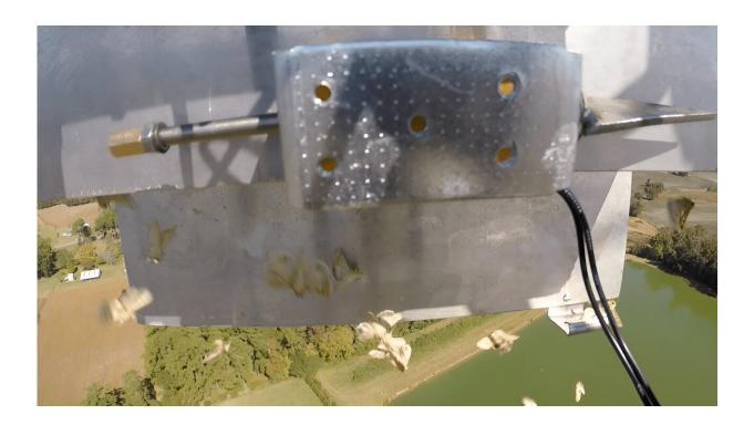
Moths were dropped out of a drone in the first attempt to test whether the ceilometer could detect flying insects. Credit: North Carolina State University
