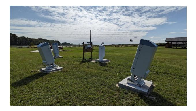
The ceilometers installed at the Tidewater Research Station are being used to detect moths and measure weather patterns. Credit: North Carolina State University
