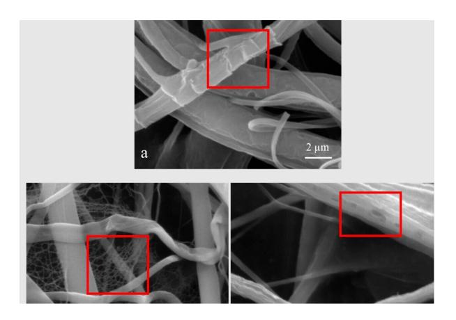
(a) PCL sponge 26 w/v%, 15 cm, 20 kV, and 10,000  $\mu$ L/h, 26 °C, 60% humidity, SEM image showing roughness of fibers. (b) SEM fibers 80:20 PCL/gel 24 w/v% on foil, 24 °C, 31% RH, 1500  $\mu$ L/h, 15 cm, 22 kV showing webbing and (c) 80:20 PCL/gel sponge 24 w/v%, 78% RH, 30 °C, 1500  $\mu$ L/h, 15 cm, 22 kV showing loss of webbing and fiber porosity. Images were taken with a field view of 15  $\mu$ m. Credit: *Nanomaterials* (2023). DOI: 10.3390/nano13243107
