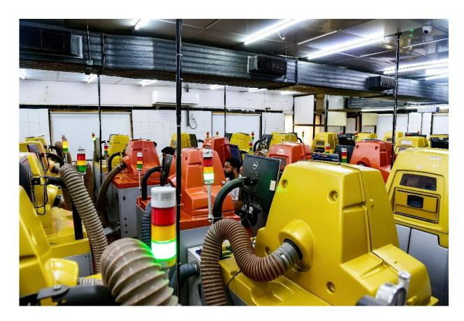
Reactors in diamond labs are pumped full of carbon-containing gases such as methane and the crystal grows under heat and pressure.
