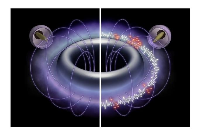
When the plasma confined in the dipole magnetic field of RT-1 contains a significant ratio of high-temperature electrons (red particles), the spontaneous formation of a chorus emission (white emission lines) is characterized by a variable frequency (sound height) like birdsong. Credit: National Institute for Fusion Science
