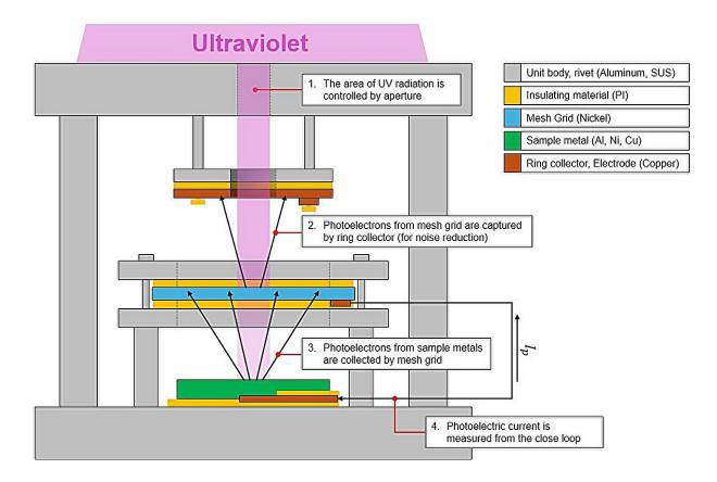
Diagram showing principle of designed measurement unit with description (not to scale). Credit: Korea Institute of Civil Engineering and Building Technology(KICT)
