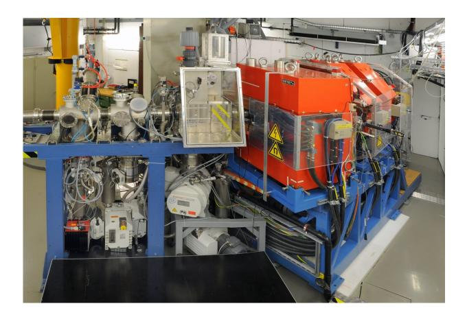
The TASCA recoil separator at GSI/FAIR in Darmstadt used for the production and isolation of superheavy elements. Credit: G. Otto, GSI/FAIR
