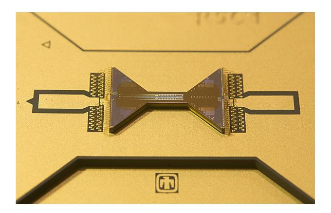
Image shows the ion trap used to control the location of computational and refrigerant ions. The device was produced by Sandia National Laboratories. Credit: Sandia National Laboratories.
