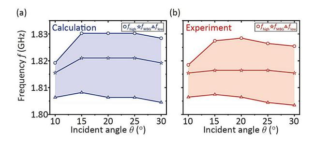
Fig. 3. A summary of the results obtained in Figure 2, with the angle of the twodimensional magnonic crystal on the horizontal axis and the magnonic band gap on the vertical axis. The calculations in (a) and the experiments in (b) are in good agreement, showing a small frequency shift and excellent performance. Credit: Taichi Goto et al
