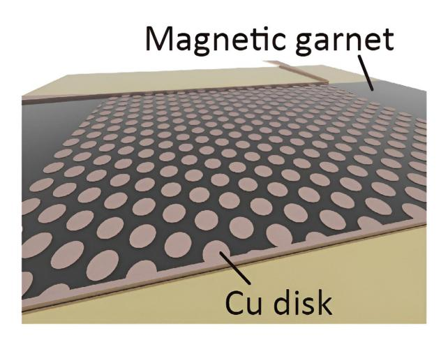
Fig. 1. An illustration of the two-dimensional magnonic crystal developed in this study, viewed from an oblique angle. Copper disks are periodically arranged on a magnetic garnet film. Credit: Taichi Goto et al
