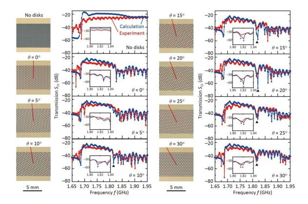
Fig. 2. Top-view photograph of the fabricated two-dimensional magnonic crystal and the spin wave transmission spectrum at that time. Even when the two-dimensional magnonic crystal is rotated by 5 degrees at a time, it can be seen that the frequency of the magnonic band gap indicated by  $\blacktriangle$  remains almost unchanged. This suggests a low angular dependence and the potential for controlling the propagation direction of spin waves. Credit: Taichi Goto et al
