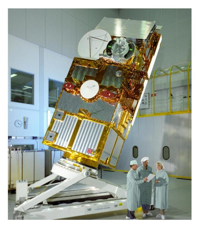
ERS-2 satellite prior to launch. ERS-2 was launched in 1995, following its sister, the first European Remote Sensing satellite ERS-1, which was launched in 1991. The two satellites were designed as identical twins with one important difference – ERS-2 included an extra instrument to monitor ozone levels in the atmosphere. Credit: European Space Agency
