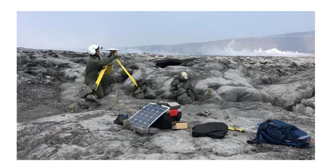
Geophysicists installed additional continuous GPS stations around Halema'uma'u this morning. These stations will allow scientists to better monitor and measure the ongoing subsidence of Halema'uma'u and the adjacent caldera floor. Credit: USGS
