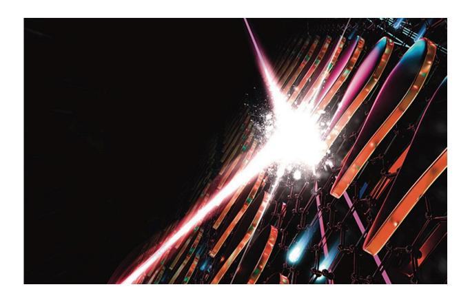
Gold nanoantennas concentrate light waves into intense nanoscale "hot spots," which excite electrons within an underlying atomically thin graphene layer. The asymmetric structure then points the electrons along a specific direction, driving electrical currents that are controllable and tunable at nanometer scales. Credit: Julia Chen
