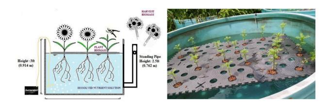
Diagram illustrates mesocosm dimensions and design (left). The picture shows a floating treatment wetland in mesocosm with cut-flower planted treatment spaced at 9 plants per m<sup>2</sup> (right). Credit: *Environmental Advances* (2023). DOI: 10.1016/j.envadv.2023.100405
