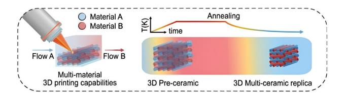
Multimaterial composition sketch representing a microfluidic cell. After printing and development, the precursor for glass/ceramic is exposed to be annealed. Credit: *Trends in Chemistry* (2024). DOI: 10.1016/j.trechm.2023.12.005
